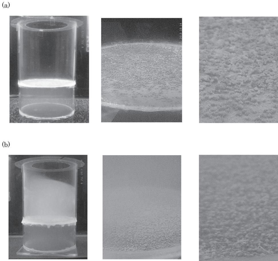
**Fig. 7.** Absence of white-turbid layer above the model aquatic sediment after 7 days of culture with  $20 \text{ mg/cm}^2$  of nutritional granule (a), and the biofilm and the white-turbid layer above the model aquatic sediment after 7 days of culture with  $10 \text{ mg/cm}^2$  of nutritional granule (b).
