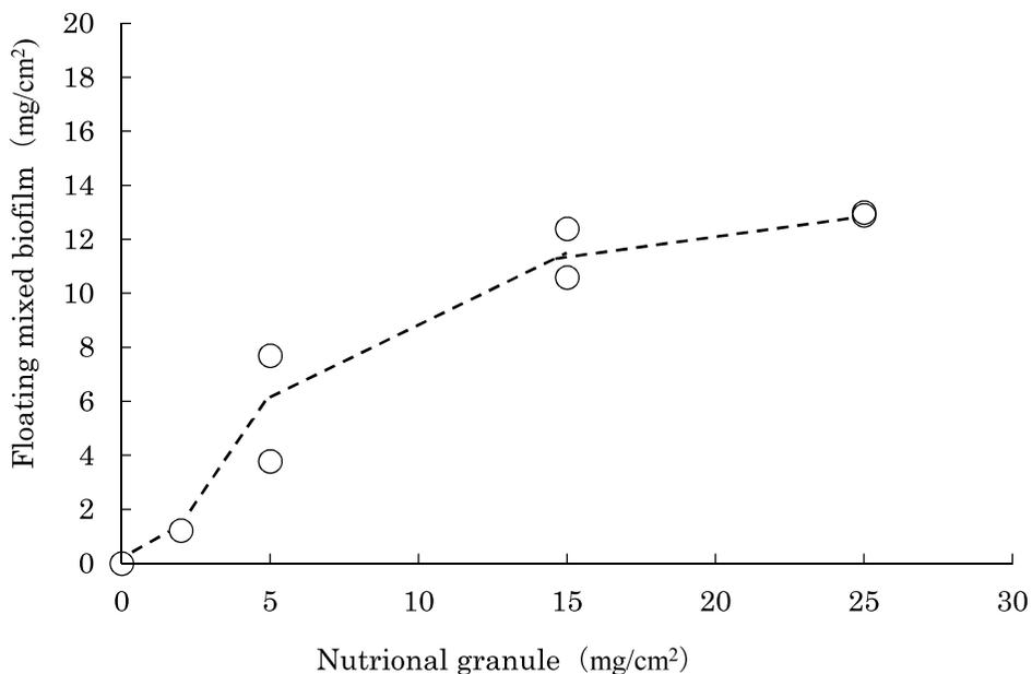
**Fig. 3.** Formation of floating mixed biofilms nourished with different amounts of nutritional granules. The weights of the floating biofilms after 7 days of culture at 20 °C are shown.
