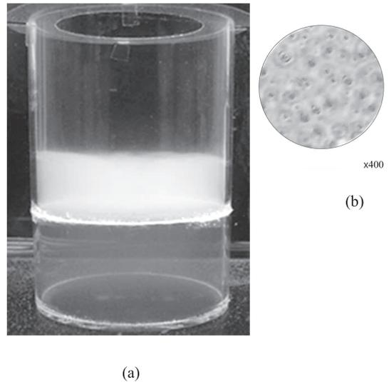
Fig. 4. White-turbid layer above the bottom of the modeled aquatic benthic boundary with biofilm growth after 5 days of culture at 20 °C (a), and a microscopic image of bacteria in the white-turbid layer (b).
