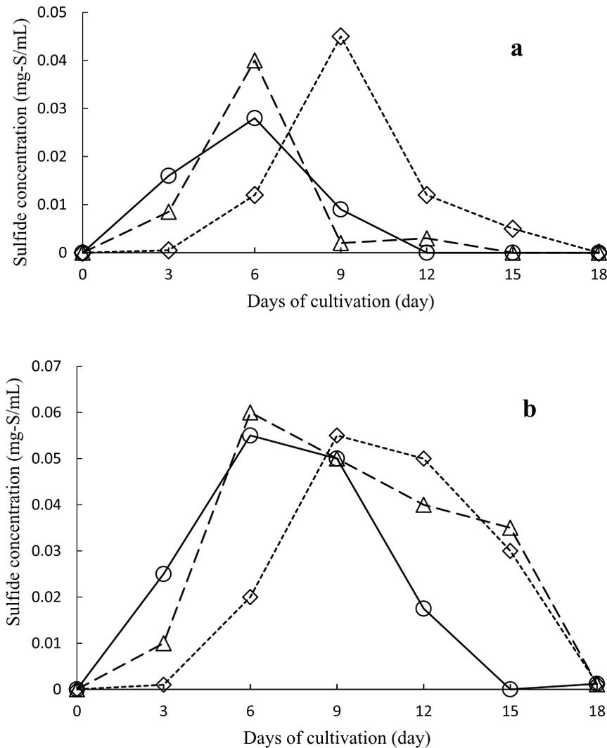
**Fig. 8.** Sulfide concentration in the water above (a) and below (b) the bottom of the aquatic benthic boundary model (nutritional granules,  $5 \text{ mg/cm}^2$ ) with biofilm growth at different water temperatures. Circles,  $25 \text{ }^\circ\text{C}$ ; triangles,  $20 \text{ }^\circ\text{C}$ ; squares,  $15 \text{ }^\circ\text{C}$ . The original sediment was collected under the TENNOZU Bridge.
