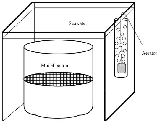
**Fig. 1.** Experimental model of biofilm formation at the aquatic benthic boundary. The model bottom (nylon mesh, 50  $\mu\text{m}$ ) was affixed in a transparent acrylic vessel (diameter, 9.5 cm; height, 15 cm) with a closed bottom and an open mouth. The acrylic vessel was submerged in a glass chamber of dimensions 18 cm (D)  $\times$  30 cm (W)  $\times$  24 cm (H).
