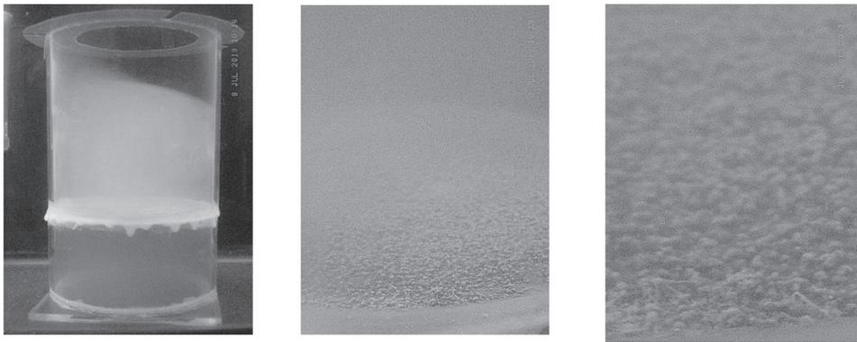
**Fig. 7.** Absence of white-turbid layer above the model aquatic sediment after 7 days of culture with 20 mg/cm<sup>2</sup> of nutritional granule (a), and the biofilm and the white-turbid layer above the model aquatic sediment after 7 days of culture with 10 mg/cm<sup>2</sup> of nutritional granule (b).
