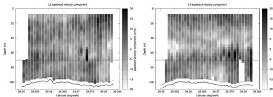
Fig. 2 Eastward velocity component ( $u$ ) sections at the first half (left) and just before the end (right) of flood tide on 30 July 2015.  $U$  above and below 70 m depth are measured by shipboard ADCP and V-fin, respectively.
